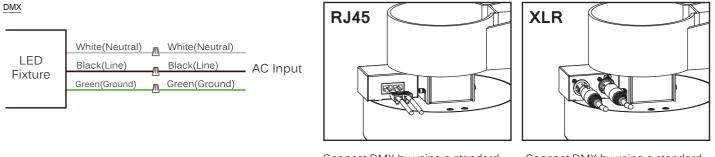
Connect DMX by using a standard shielded CAT5/6 cable.
