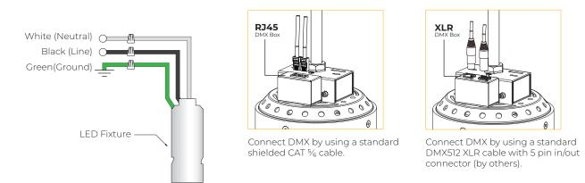
\*The last fixture has to be terminated with a DMX Terminator (by others).
