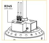
Connect DMX by using a standard shielded CAT % cable.
