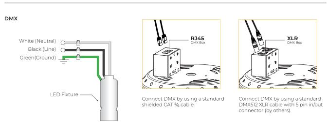
\*The last fixture has to be terminated with a DMX Terminator (by others).
