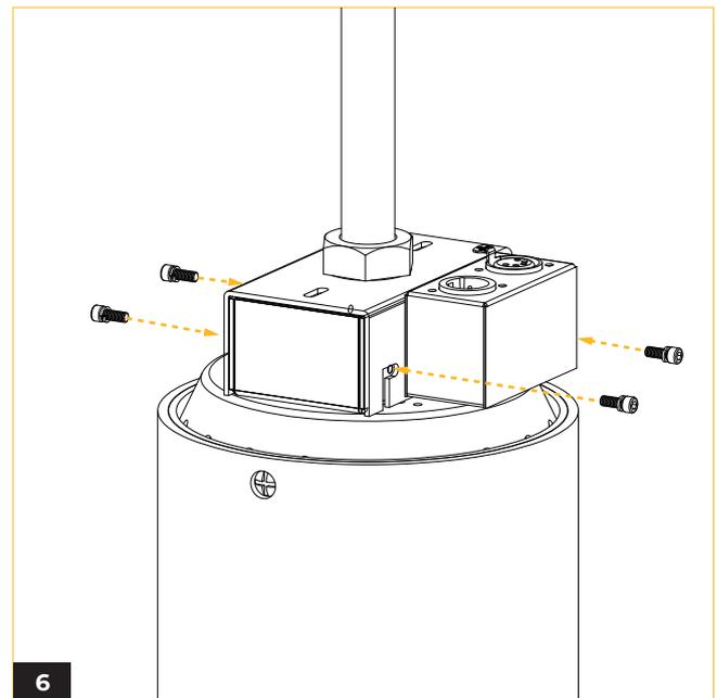
Screw four Phillips screws to fasten the mounting bracket on the wiring box.
