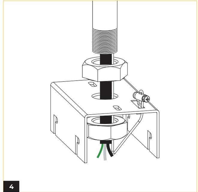
Place two screw nuts on either side of the mounting bracket, making sure the safety cable is also placed through. Loop and fasten the safety cable through the slot available on the mounting bracket.
