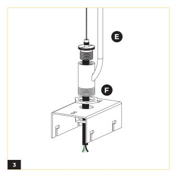
(E) Insert the cable through the gripper and plunger. Trim off extra cable using cable cutting tool. To adjust the cable to desired length, press the plunger.
