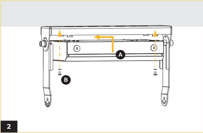
**(A)** Slip the power box hook with fastener over the lock-in grooves allocated.
