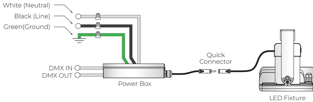
**\*The last fixture has to be terminated with a DMX Terminator (by others).**
