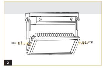
Secure the fixture to the bracket with provided screws and establish electrical connections. (Refer to wiring diagram)
