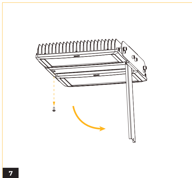
7 Open twin lighthouse junction box to expose stem opening.
