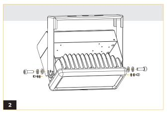
Slip the power box hook with fastener over the lock-in grooves allocated and fasten screws on either side to keep the power box in place.
