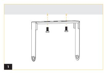
Secure bracket to a level surface with mounting hardware that is sufficient to support weight of the fixture and power box.
