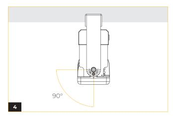
The light engine can be adjusted within a range of ±90 degrees. To secure the rotated position, tighten the screws on each side.
