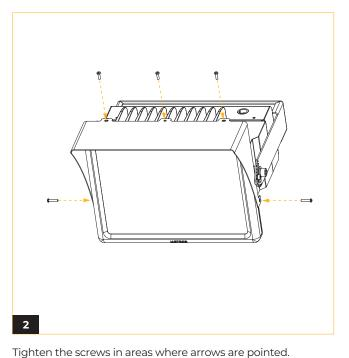
Put the shield on the fixture.
