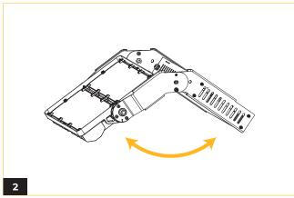
Unfold the luminare body until the screw points are aligned.
