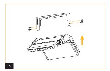
Align the bracket with the luminaire body, and fasten the bracket by using two screws on each side. Ensure that the unfolded body is also securely fixed and remains stable.
