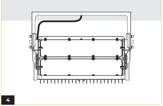
Establish electrical connections between the junction box and the fixture. (Refer to wiring diagram)
