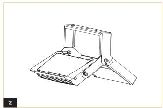
Align the Glare Shield Visor with the light engine and secure it in place by fastening the corresponding screws.
