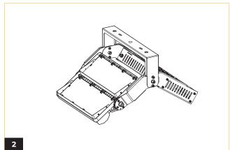
Align the Glare Shield Visor with the light engine and secure it in place by fastening the corresponding screws.
