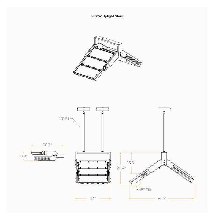
BOLT NOVA NEXT GEN NATATORIUM-RATED INDIRECT LUMINAIRE
