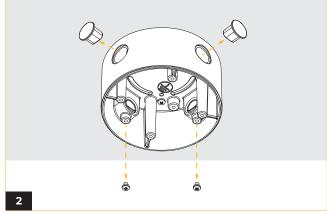
Remove the screws from the bottom of the junction box to release the conduit end caps.
