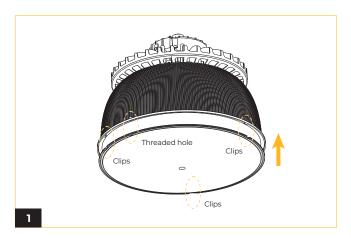
Locate the clips and threaded hole to matching positions.
