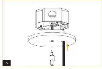
Thread the power cord and dimming wires through the canopy wire hole.
