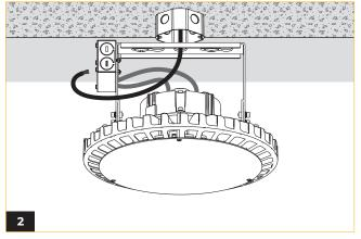
Make electrical connections between junction box according to the wiring diagram.
