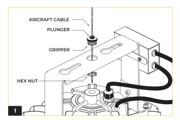
Insert the cable through the gripper and plunger. Press the plunger to adjust the cable to desired length.
