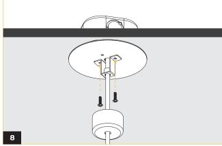
Fasten canopy plate in place using 2 phillips screws.
