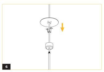
Thread wires though canopy mount, bracket and plate.
