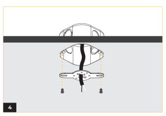
Secure the crossbar to junction box (by others), using two phillips screws.
