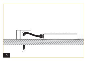
Thread the DC cables from powerbox through the junction box.  $\label{eq:cables}$
