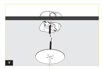
Make electrical connections between crossbar and mounting plate. Refer to the wiring diagram for more detailed instructions.
