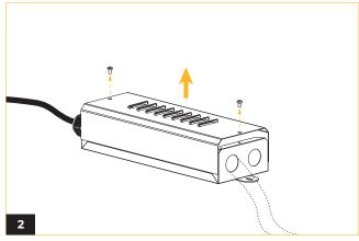
Remove powerbox lid to make electrical connections (Refer to wiring diagram).
