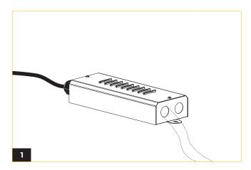
Remove knockout for power connection.
