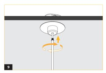
Fasten stem on canopy mount by rotating clockwise.
