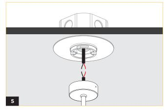
Make electrical connections between junction box and luminaire. Refer to the wiring diagram for a more etailed explanation.
