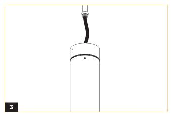
Thread luminaire wiring through stem mount.
