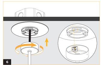
Raise and align the stem mount canopy to the plate by matching the U-shaped openings.
