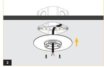
Screw the stem adjustable mount plate onto the bracket in the two holes indicated.
