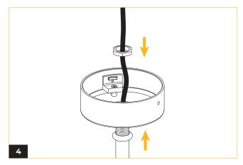
Fasten stem mount canopy and fasten in place using hex nut.
