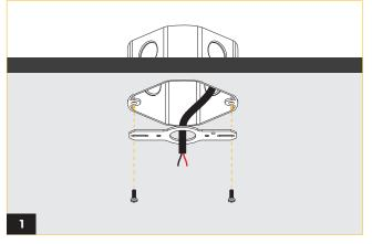
Secure the crossbar to junction box (by others), using two phillips screws.
