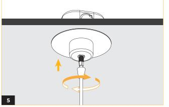
Screw in the cord grip cap to finish the installation.
