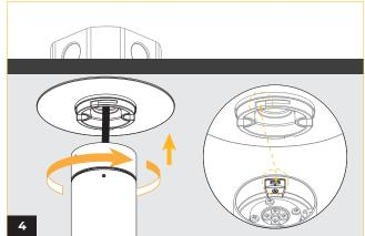
Align the bottom part of the fixture with the surface mount plate by matching the U-shaped openings.
