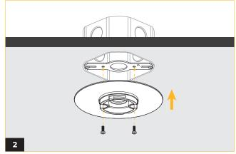
Screw the surface adjustable mount plate onto the bracket in the two holes indicated.
