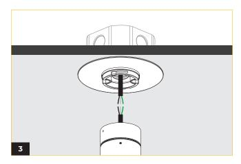
Refer to the wiring diagram for connection to the junction box.  $\label{eq:connection}$
