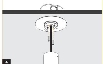
Secure top cover of luminaire to canopy plate using 2 phillips screws
