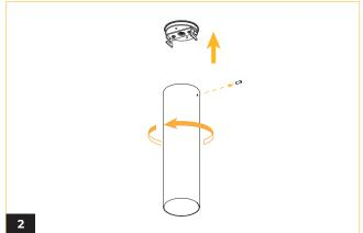
Remove top cover of luminaire by removing the hex screw located on the side of the luminaire.
