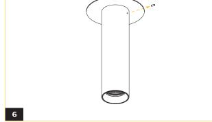
Secure the luminaire onto the top cover by hoisting level and rotating clockwise.
