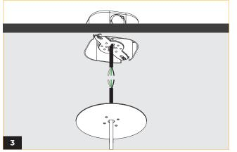
Make electrical connections between crossbar and mounting plate. Refer to the wiring diagram for more detailed instructions.
