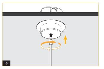
Screw in the cord grip cap to finish the installation.
