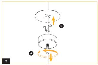
Remove the base and cap of the cord grip, adjust mounting length accordingly. Once adjusted to a desired height, slip cord through canopy plate.
