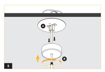
(A) Fasten canopy plate in place using 2 phillips screws.
