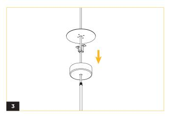
Thread wires though canopy mount, bracket and plate.
