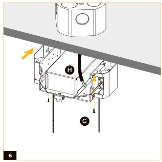
(G) Slide the power module onto the mounting plate and fasten the two screws previously removed on opposite corners of the mounting plate.
