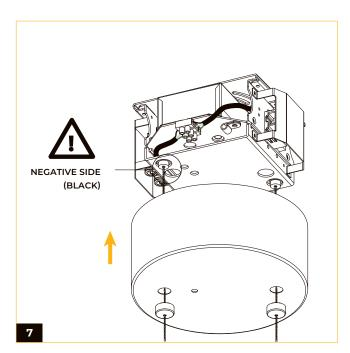
Identify the negative side of the fixture (Marked by a black discoloration and a label sticker), Place the canopy around the power module and fasten the two bolts.
