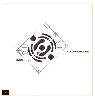
Mark an alignment line on the ceiling and align it with the indicated markers on the mounting plate. The mounting plate will be slanted at an angle in relation to the horizontal line as shown in the diagram.
