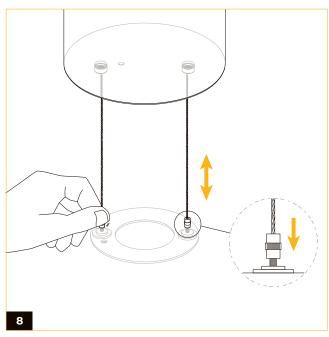
To adjust the cable gripper, simply turn it clockwise by 2-3rotations. Then push down to unclamp the wire. Note: Adjusting the height without attaching the fixture is less strenuous.
