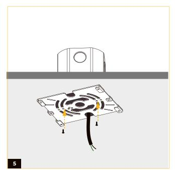
Once aligned, screw the mounting plate into place with 2-3screws on the available ports and thread through the wires from the junction box.
