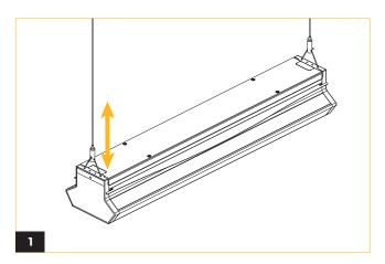
Continue the installation by following one of the previously outlined ceiling mounting methods. Insert the aircraft cable through the gripper and plunger assembly, then adjust the plunger to set the cable to the desired length. Ensure the cable is firmly secured before releasing.
