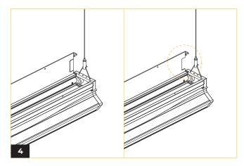
Remove the rectangular knockout on the top cover to create clearance for wiring where needed.
