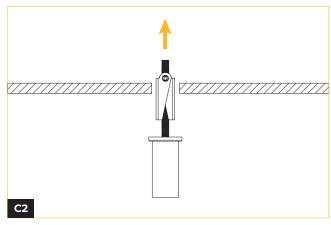
Insert the toggle bolt through the coupler, then pass the assembly through the ceiling opening.
