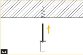
Insert the screw through the coupler and drive it into the drywall anchor. Ensure the screw is fully tightened for a secure installation.
