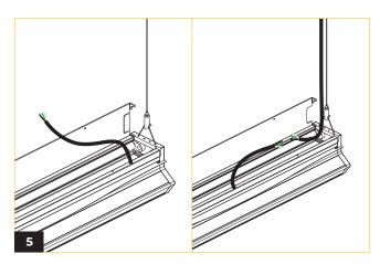
Guide the power cables through and make the electrical connections to the fixture's internal wiring (refer to the wiring diagram). Ensure all connections are properly secured.
