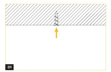
Drill the self-drilling drywall anchor into the ceiling. Ensure the anchor is firmly secured and flush with the surface.
