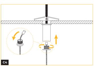
Feed the aircraft cable through the coupler until the terminal locks securely into place. Screw in the assembly to confirm a firm and secure fit.
