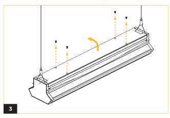
Remove the four screws and swing open the hinged top cover to access the internal components.
