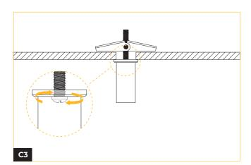
Tighten the screw firmly to secure the coupler against the ceiling surface.
