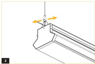
Tighten the lower adjustment screw to ensure the fixture remains level and balanced.
