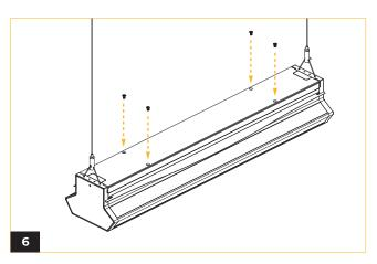
Close the top cover and secure it in place with screws.
