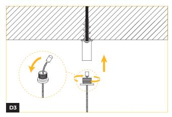
Feed the aircraft cable through the coupler until the terminal locks securely into place. Screw in the assembly to confirm a firm and secure fit.
