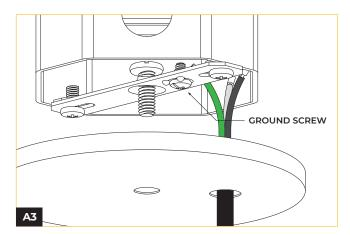
Connect the ground conductor to the ground screw on the crossbar, then connect the line and neutral wires according to the wiring diagram.
