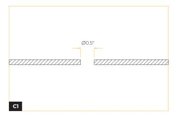
Cut a 0.5 inch hole in the ceiling. Ensure the hole is clean and free of debris before proceeding.
