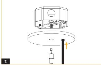
Thread the power cord and dimming wires through the canopy wire hole.
