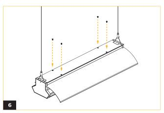
Reinstall the top caReinstall the top covers and secure it in place with screws.
