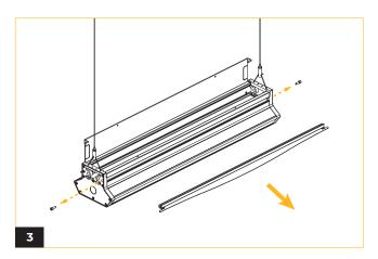
Loosen the mounting screws securing the diffuser, then carefully detach the diffuser from the fixture.
