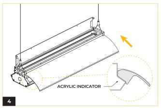
Slide the downlight blade into the groove, using the acrylic indicator to position it at the correct angle.
