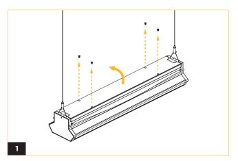
Remove the four screws and swing open the hinged top cover to access the internal components.
