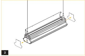
Remove the front and rear cover plates, which are held in place by magnets.
