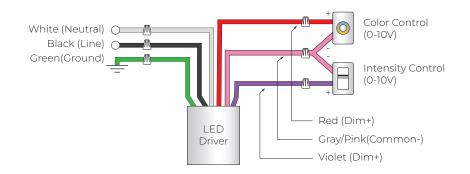
**REV 4** WIRING DIAGRAM
