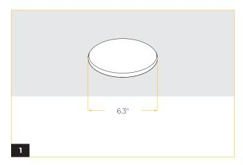
Mark the intended location of the luminaire and cut an 6.3"(160mm) diameter opening in the ceiling.
