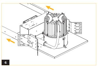
Install fixture using universal mounting bracket with slots for C-Channel (by others), bar hanger (by others) and 1/2" EMT (by others). Secure to joist or grid using hardware or wire. Adjust height as needed.
