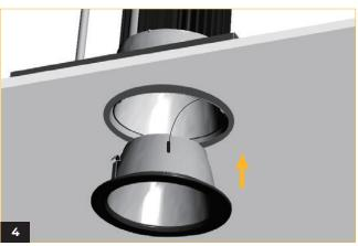
Connect safety cable to trim and push reflector into the frame to ensure the trim is flush to the ceiling.
