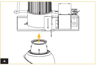
Secure the safety wire and push the trim and reflector back into the fixture.
