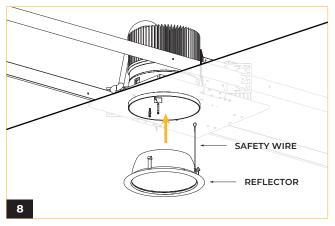
Connect safety wire and push reflector into frame ensuring the trim is flush to the ceiling.
