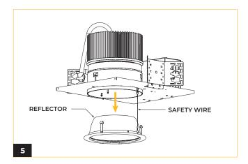
Separate the reflector from the fixture by pulling down.
