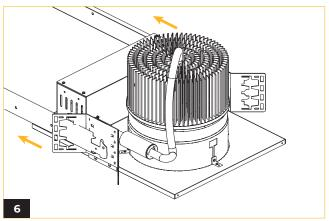
Install fixture using universal mounting bracket with slots for C-Channel (by others), bar hanger (by others) and 1/2" EMT (by others). Secure to joist or grid using hardware or wire. Adjust height as needed.
