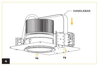
An optional handlebar can be installed to assist the installation process, secure the handle bar by screwing in two screws on each side.
