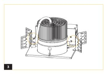
Secure the butterfly bracket by screwing in the provided wing  $\operatorname{nut}$ .
