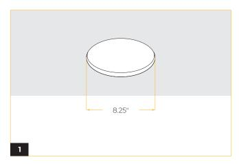
Mark the intended location of the luminaire and cut an 8 1/4" diameter opening in the ceiling.
