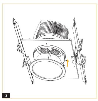
Connect safety cable to trim and push reflector into the frame to ensure the trim is flush to the ceiling.
