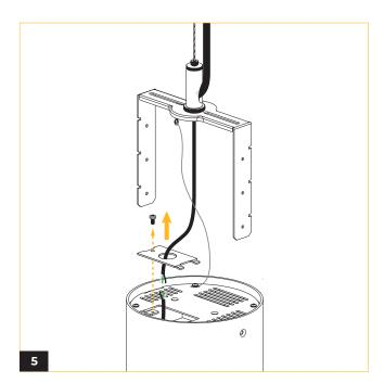
Remove the power feed lid to expose the power cord, route the wiring from the power source through the lid, and make electrical connections as shown in the wiring diagram.
