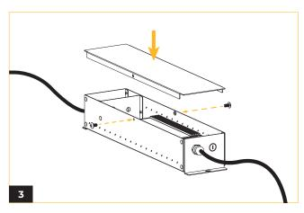
Reattach the power box cover by aligning it properly and securing it with the two screws on each side.
