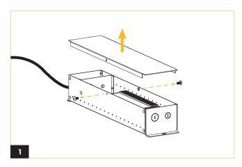
Remove the power box cover by unscrewing the two screws on each side.
