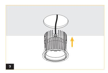
Install the downlight by inserting it through the ceiling cutout.
