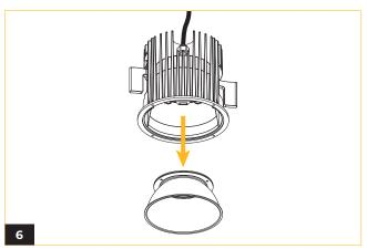
Detach the reflector from the fixture by carefully pulling it away from the magnets.
