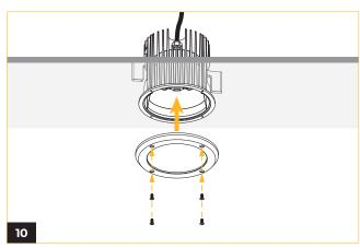
Reattach the glass trim cover by aligning it with the fixture and securing it with the four front screws.
