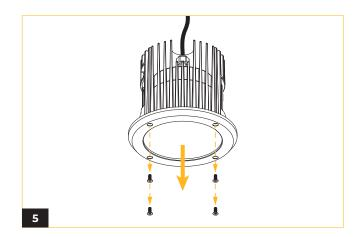
Remove the glass trim cover by unscrewing the four front screws.
