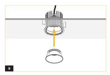
Reattach the reflector by aligning it with the fixture and securing it onto the magnets.
