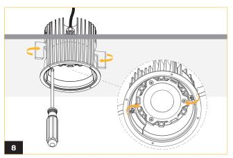
Using a screwdriver, tighten the screws to expand the two side brackets, securing the fixture firmly in place.
