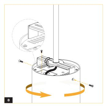
Install the fixture onto the bracket by aligning the slots, twisting the fixture counterclockwise until locked, and securing it with two screws on each side.
