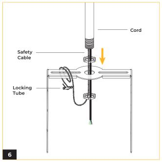
Insert the safety cable and wiring through the stem, then slide the stem through the bracket and secure it by tightening the nuts on both sides. Loop the safety cable around the bracket, secure it with the locking tube, and tighten the screws to hold it in place.
