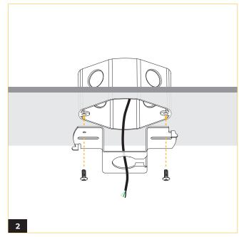
Attach swivel crossbar to junction box (not included) with two screws.
