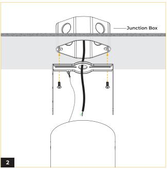
Mount the bracket to the desired location and secure it to the junction box (not included) using appropriate hardware.
