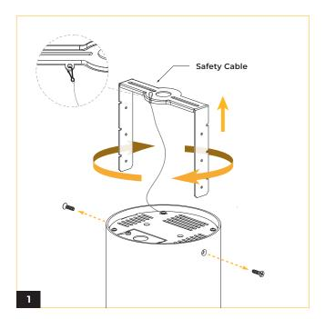
Remove the bracket by unscrewing the two screws on each side of the fixture, then twist it clockwise to detach.
