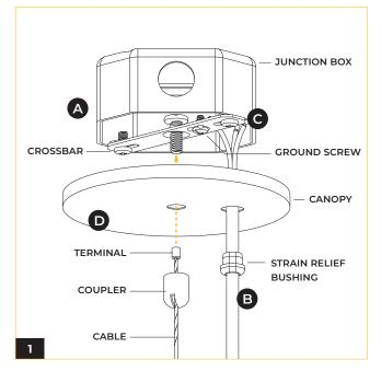
(A) Secure the crossbar to the 4" octagonal box (by others) designed to support the weight of the fixture.
