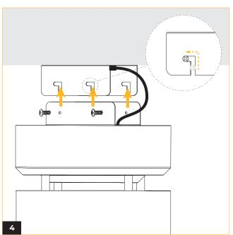
Screw 4 phillips screws to secure the wiring box on the mounting bracket. Lock and latch onto the mounting bracket, and tighten in place once secured.
