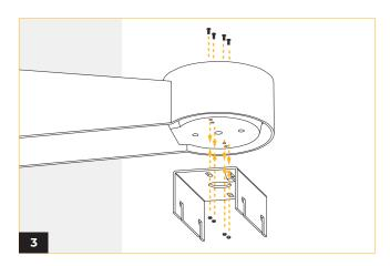
Secure the mounting bracket to the wall mount with the provided screws.
