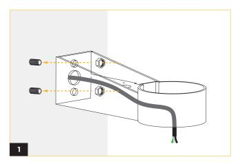
Secure wall mount to surface with mounting hardware (by others) that is sufficient to support weight of fixture. Route AC cable through center hole on wall mount.
