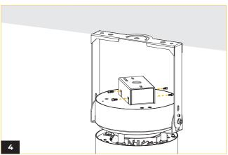
Screw 4 phillips screws to secure the wiring box.
