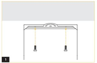
Secure Yoke Mount to surface with mounting hardware (by others) that is sufficient to support the weight of the fixture.
