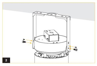
Loosen four Phillips screws on the side of the wiring box to remove the mounting bracket.
