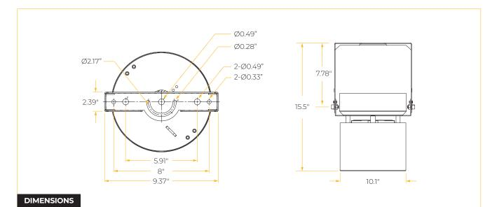
Secure Yoke Mount to surface with mounting hardware (by others) that is sufficient to support the weight of the fixture.
