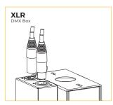
Connect DMX by using a standard DMX512 XLR cable with 5 pin in/out connector (by others).
