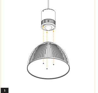
Bring shroud to the fixture level and align it to the indicated openings. Fasten shroud in place with three phillips screws.
