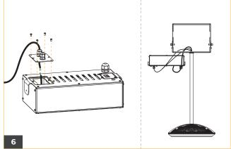
Unscrew the DC junction box and loosen the cable clamp. Insert the DC wire through the cable clamp and connect them to the wires in the junction box. After connection, ensure firmness by tightening cable clamp. Connect the RJ45 connector to the port on the power box. Refer to the wiring diagram for a detailed explanation.
