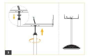
Slot through the RJ45 connector and DC cables through a Hex screw and tighten the Hex screw on the stem grooves.
