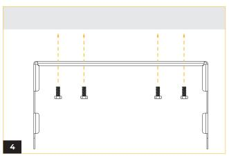
Fasten the top bracket on the desired location on the ceiling.
