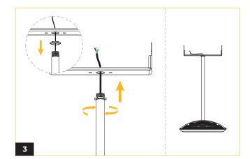
First, push the cables through a Hex screw and tighten on stem grooves. Second, fasten the stem onto the lower bracket.
