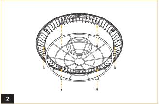
Align the attachment in place and secure it firmly by tightening the screws.
